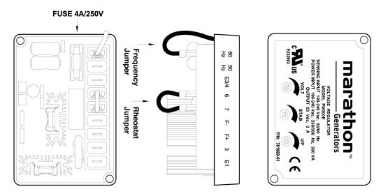
Figure 2 Jumper and Potentiometer Control Locations
