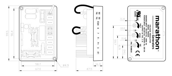
Figure 1 Outline and Drilling Diagram
