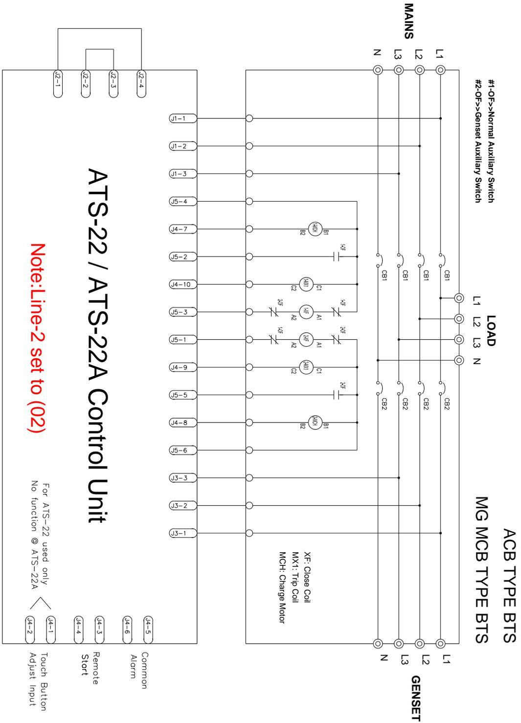
**5.8 Air Circuit Breaker Type ATS Wiring Diagram (2P 220 Vac)**
