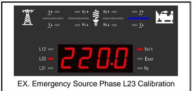
Step 4 : Use a good quality voltmeter as a reference to calibrate the ATS-22A voltage reading to the desired phase.
