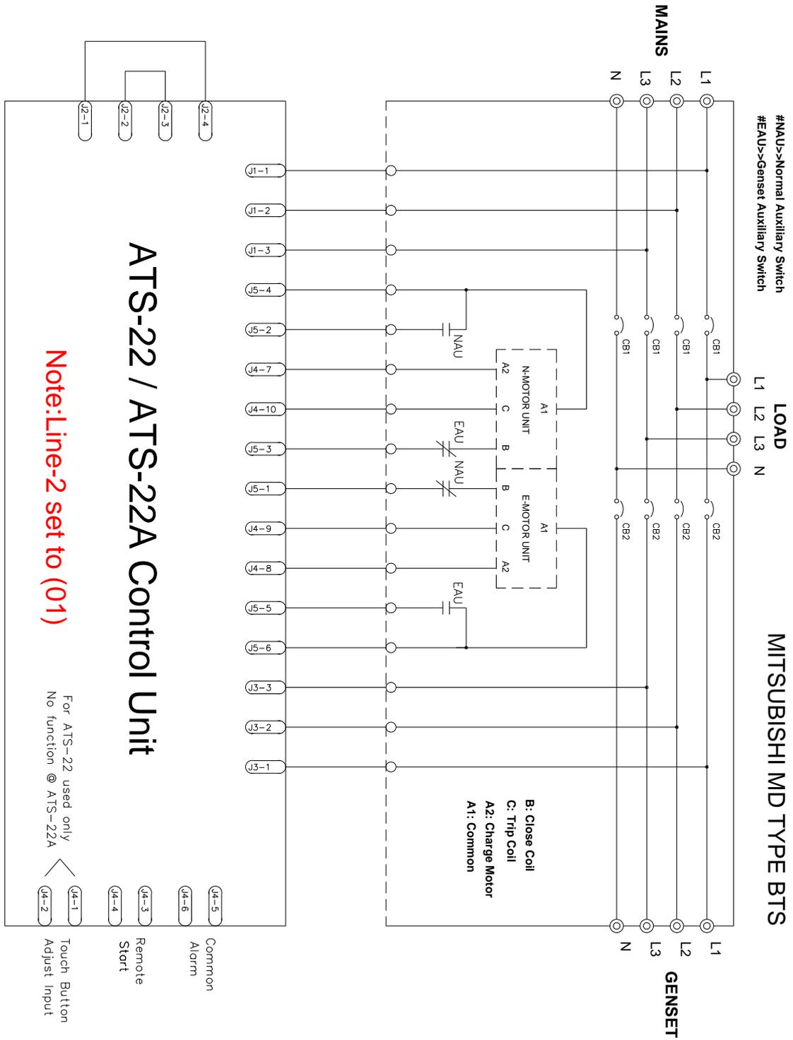
5.6 MITSUBISHI MD Type ATS Wiring Diagram (2P 220 Vac) – MCCB With Separate Motor
