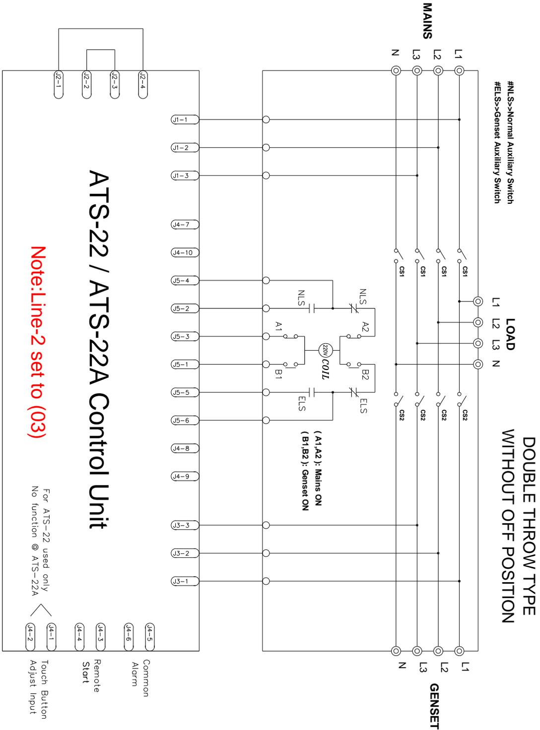
5.10 Double Throw Type ATS Without OFF Position Wiring Diagram (2P 220 Vac) – With A1, A2 & B1, B2
