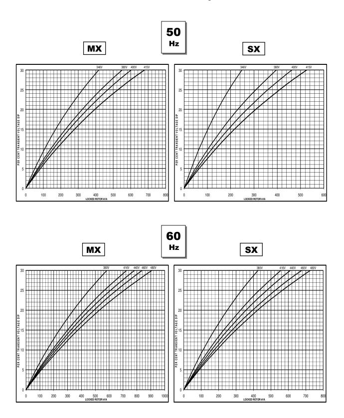
Three-phase Short Circuit Decrement Curve. No-load Excitation at Rated Speed Based on star (wye) connection.
